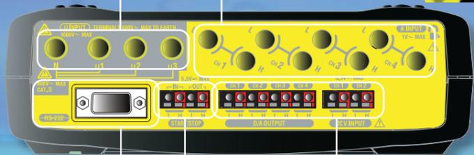
RS-232 connector External control input/output Analog input/output terminal (optional)
